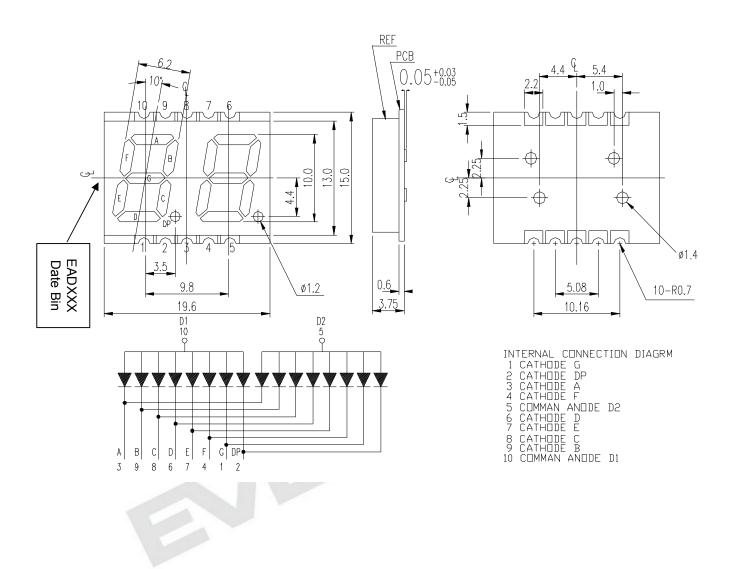
Note: Tolerances unless mentioned ±0.25mm. Unit = mm
