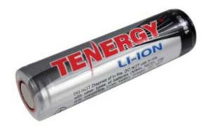
This is a rechargable Li-ion Cell in an "18650" form factor. Made by Tenergy, this cell is rated at 3.7 V and 2600 mAh. This is a "protected" type of lithium cell, with a built in PCB. Pair these with our Small Robot Pack-Charger to provide long-lasting, consistent power for your Boe-Bot, Shield-Bot or ActivityBot robot.
