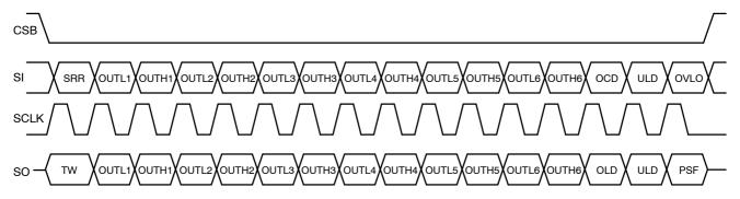
Figure 3. SPI Communication Frame Format
