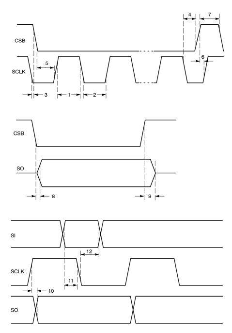
Figure 2. SPI Timing Diagram
