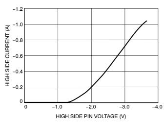
Figure 6. Typical High-side Negative Clamp Voltage vs. Reverse Current, Room Temperature
