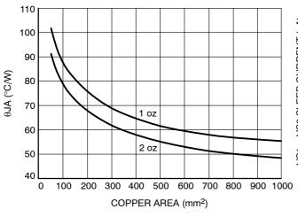
Figure 8. θJA vs. Copper Spreader Area
