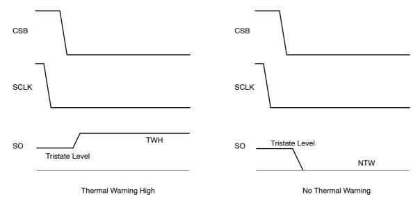
Figure 4. Access to Temperature warning information shows the thermal information is available immediately with activation of the CSB signal without having to toggle the SCLK line.
