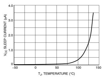
Figure 7. V<sub>CC</sub> Sleep Supply Current vs. Temperature
