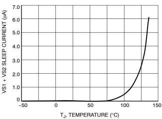
Figure 9. VS1 + VS2 Sleep Current vs. Temperature
