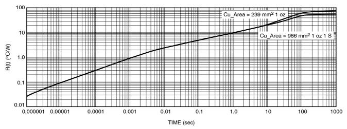
Figure 10. SOIC 28-Lead Single Pulse Heating Curve
