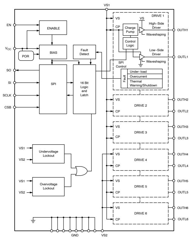
Figure 1. Block Diagram
