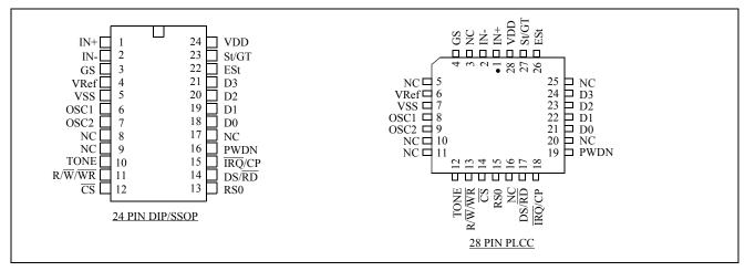
Figure 2 - Pin Connections
