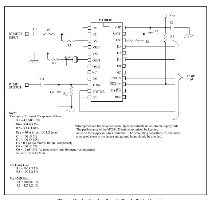
Figure 13 - Application Circuit (Single-Ended Input)
