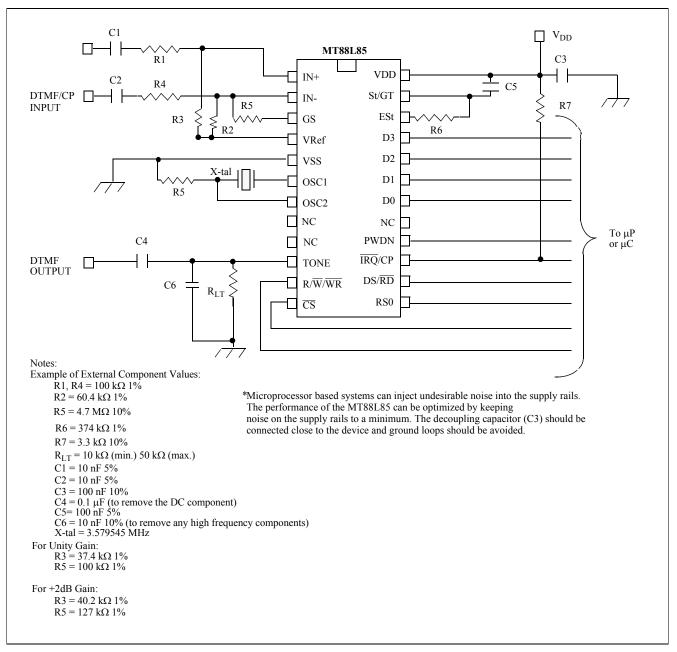
Figure 14 - Application Circuit (Differential Input Configuration)
