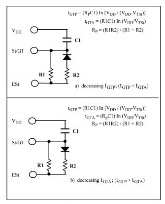
Figure 6 - Guard Time Adjustment
