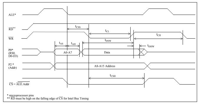
Figure 19 - Intel Write Timing Diagram
