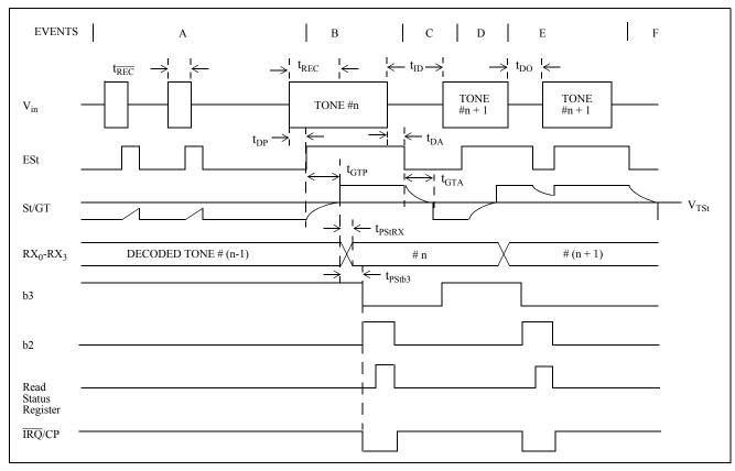
Figure 7 - Receiver Timing Diagram
