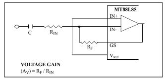
Figure 3 - Single-Ended Input Configuration
