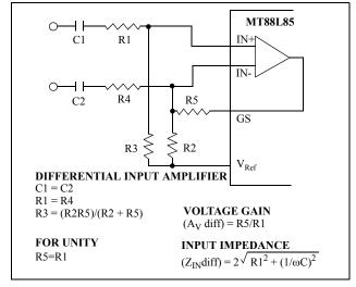
Figure 4 - Differential Input Configuration
