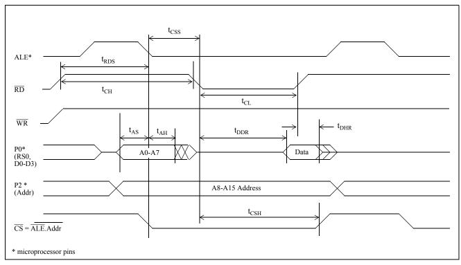
Figure 18 - Intel Read Timing Diagram
