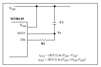
Figure 5 - Basic Steering Circuit
