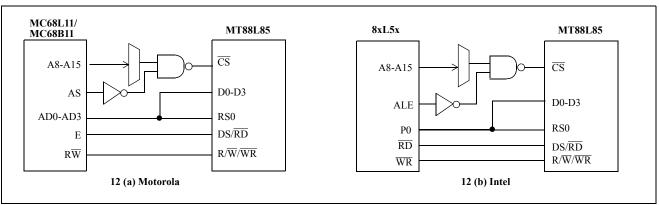
Figure 12 a) & b) - MT88L85 Interface Connections for Various Intel and Motorola Micros
