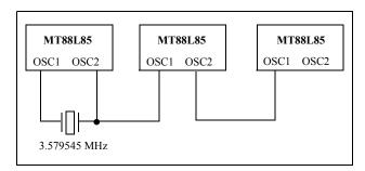
Figure 11 - Common Crystal Connection
