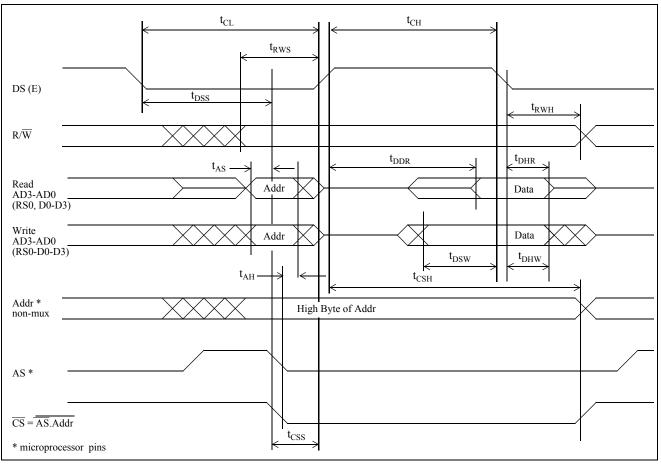
Figure 17 - Motorola BUS Timing Diagram
