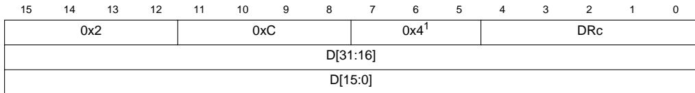
Figure 5-42. WDMREG BDM Command Format
