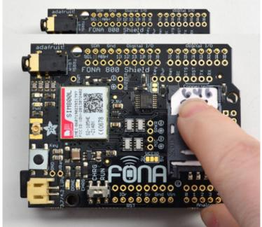
Close the hinge down and slide the cover to lock it in place
