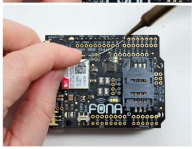
Be sure to solder all pins for reliable electrical contact.
