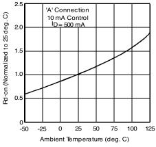
Figure 4. Typical Normalized On-Resistance
