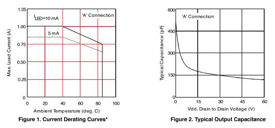
\* Derating of 'B' and 'C' connection at +85°C will be 70% of that specified at +40°C and is linear from +40°C to +85°C.
