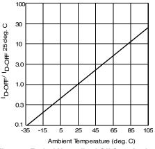
Figure 5. Typical Normalized Off-State Leakage
