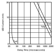
Figure 7. Typical Delay Times
