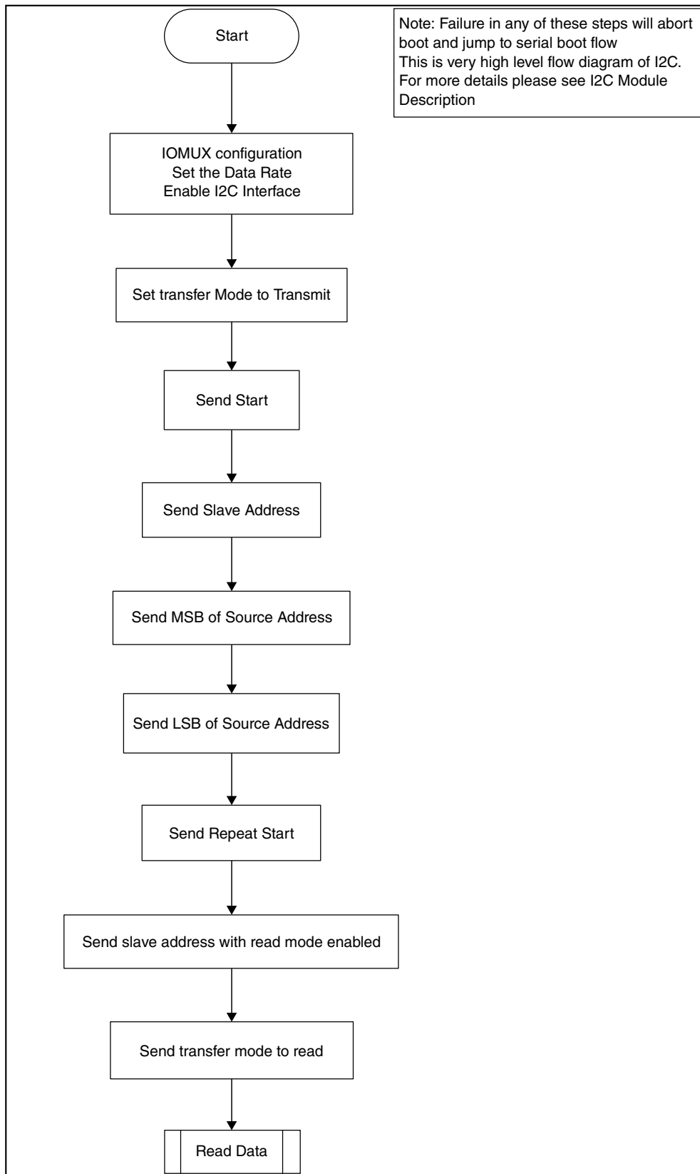
Figure 19-5. I2C Boot Flow Diagram
