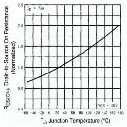
Fig. 4 - Normalized On-Resistance vs. Temperature
