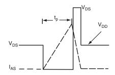
Fig. 12b - Unclamped Inductive Waveforms
