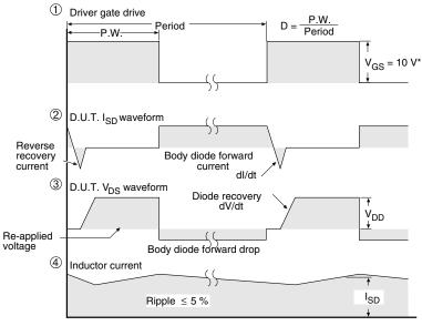
\* V<sub>GS</sub> = 5 V for logic level devices
