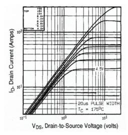
Fig. 2 - Typical Output Characteristics,  $T_C = 175$  °C
