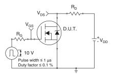
Fig. 10a - Switching Time Test Circuit
