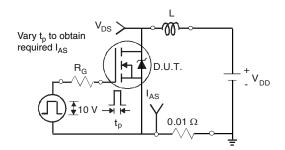
Fig. 12a - Unclamped Inductive Test Circuit
