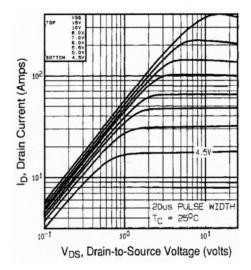
Fig. 1 - Typical Output Characteristics, T<sub>C</sub> = 25 °C
