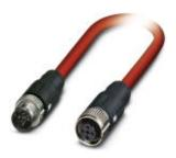
Network cable, Sercos III CAT5 (100 Mbps), 4-position, PVC/PVC, signal red RAL 3020, shielded, Plug straight M12 SPEEDCON / IP67, Coding: D, on Socket straight M12 SPEEDCON / IP67, Coding: D, Cable length: 2 m
