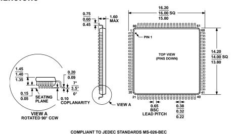
Figure 4. 80-Lead Low Profile Quad Flat Package [LQFP] (ST-80-2) Dimensions shown in millimeters
