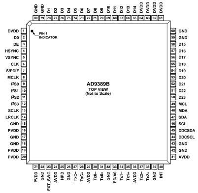
Figure 3. 80-Lead LQFP Pin Configuration (Top View)
