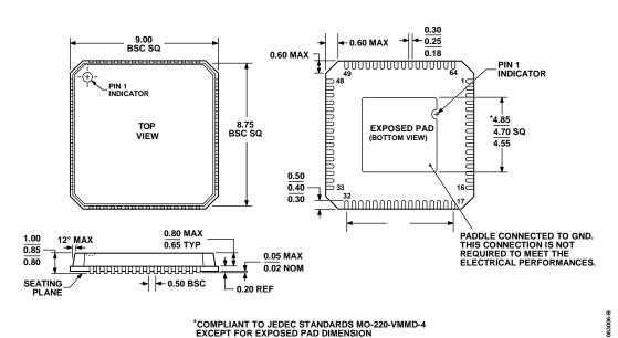
Figure 5. 64-Lead Lead Frame Chip Scale Package [LFCSP] (CP-64-1) Dimensions shown in millimeters
