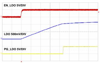
FIGURE 23. SOFT-START AT FULL LOAD, 100µs/DIV
