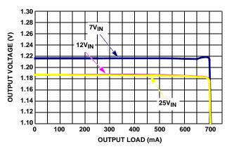
FIGURE 17. LDO vs LOAD, 500kHz,  $V_{IN}$  LDO = 3.3V
