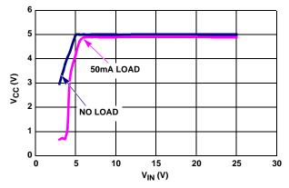
FIGURE 16.  $V_{CC}$  REGULATION WITH  $V_{IN}$
