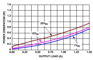
FIGURE 12. POWER DISSIPATION vs LOAD, 3.3V<sub>OUT</sub>
