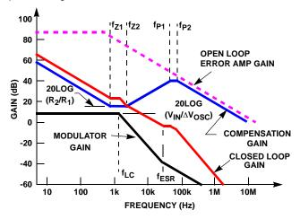
FIGURE 31. ASYMPTOTIC BODE PLOT OF CONVERTER GAIN
