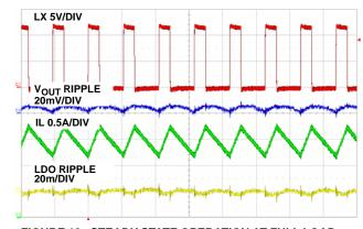
FIGURE 19. STEADY STATE OPERATION AT FULL LOAD,  $2\mu s/DIV$
