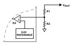
FIGURE 29. EXTERNAL RESISTOR DIVIDER
