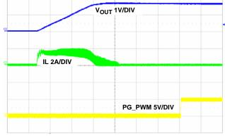
FIGURE 26. OUTPUT SHORT CIRCUIT, 5µs/DIV
