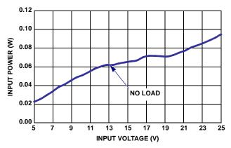
FIGURE 13. INPUT POWER vs  $V_{IN}$ ,  $V_{OUT} = 3.3V$
