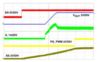
FIGURE 22. SOFT-START AT FULL LOAD, 500µs/DIV
