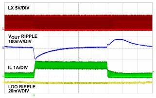
FIGURE 20. LOAD TRANSIENT, 200µs/DIV
