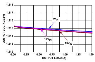
FIGURE 6.  $V_{OUT}$  REGULATION vs LOAD, 500kHz 1.2 $V_{OUT}$
