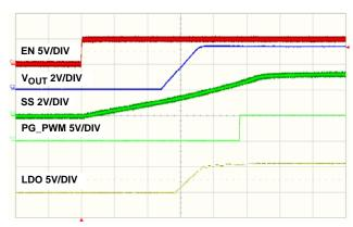
FIGURE 21. SOFT-START AT NO LOAD, 500µs/DIV
