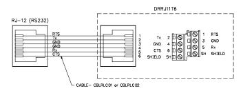
A Red Lion Controls device with an RS232 RJ-12 port is connected to the DRRJ11T6 adapter using the CBLRLC01 or CBLRLC02 cable. The terminal block is then wired to run the RS232 serial information to another device.
