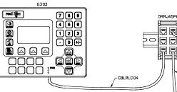
The 10' long CBLRLC04 connects the G3, which is mounted on the door of the enclosure, to the DRRJ45P6, which is located on the DIN rail next to the Modular Controllers. The 1' long CBLRLC03 cables are used to jumper from the DRRJ45P6 to the Modular Controllers.
