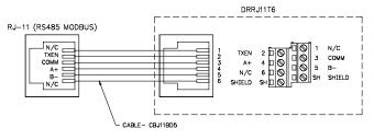
A Red Lion Controls device with an RS485 RJ-11 port is connected to the DRRJ11T6 adapter using the CBJ11BD5 cable. The terminal block is then wired to run the RS485 MODBUS serial information to another device.
