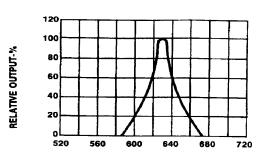
WAVELENGTH (λ)-nm Fig.2 SPECTRAL RESPONSE
