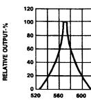
WAVELENGTH (λ)-nm Fig.2 SPECTRAL RESPONSE
