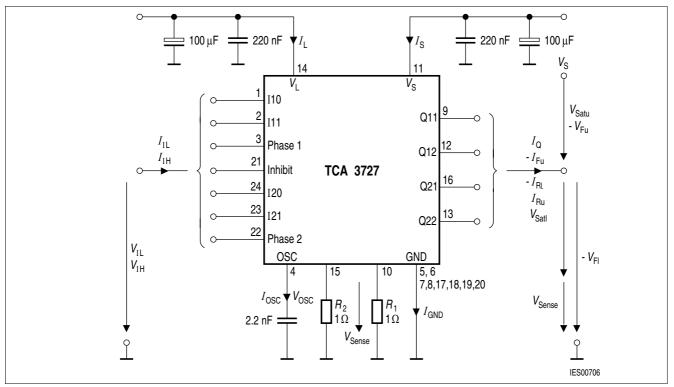
Figure 3 Test Circuit
