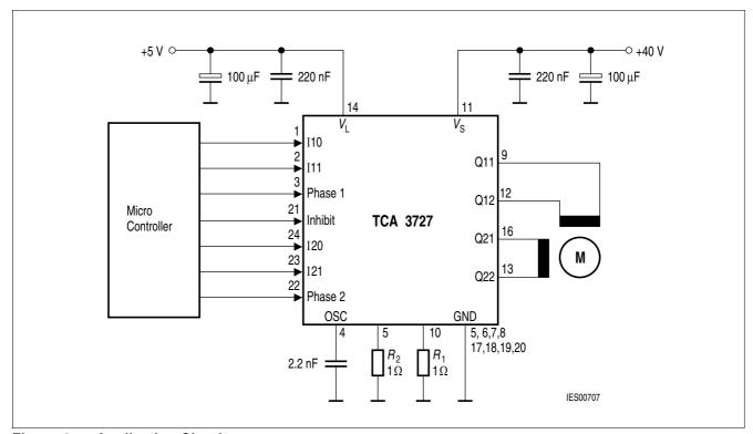
Figure 4 Application Circuit
