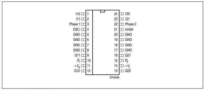
Figure 1 Pin Configuration (top view)
