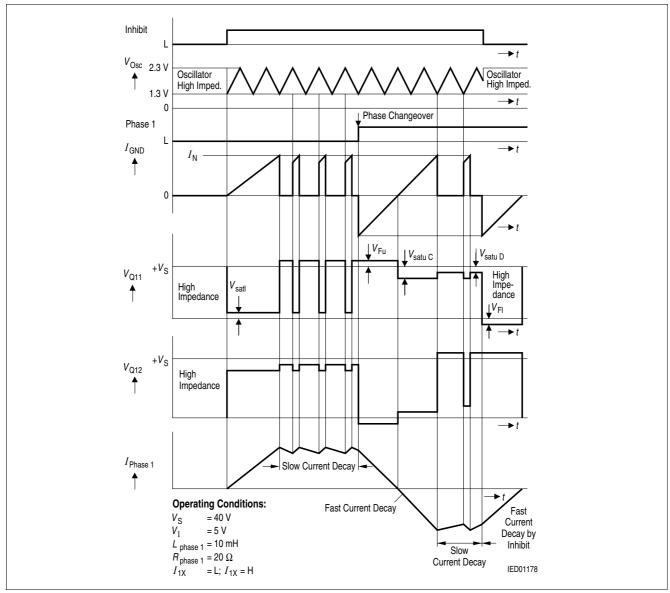
Figure 10 Phase Reversal and Inhibit
