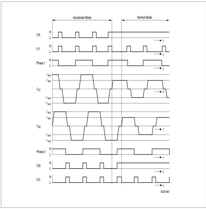
Figure 6 Half-Step Operation
