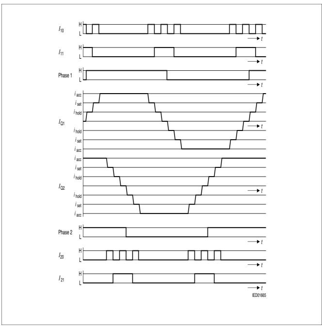
Figure 8 Mini-Step Operation
