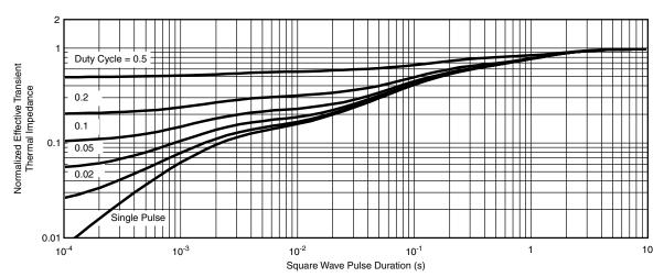
Normalized Thermal Transient Impedance, Junction-to-Foot
