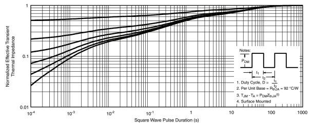
Normalized Thermal Transient Impedance, Junction-to-Ambient
