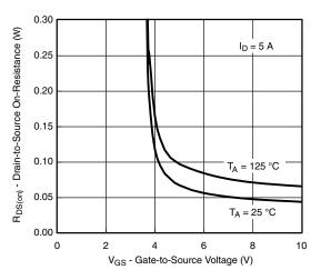
On-Resistance vs. Gate-to-Source Voltage
