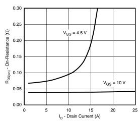
On-Resistance vs. Drain Current and Gate Voltage
