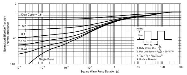
Normalized Thermal Transient Impedance, Junction-to-Ambient
