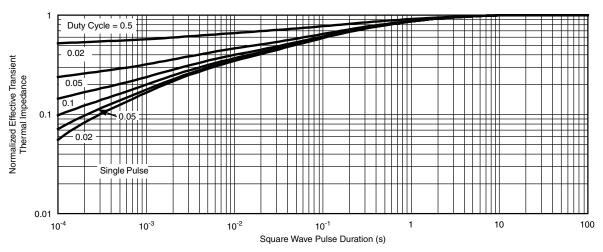
Normalized Thermal Transient Impedance, Junction-to-Foot
