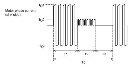
Figure 4 Motor Current Timing
