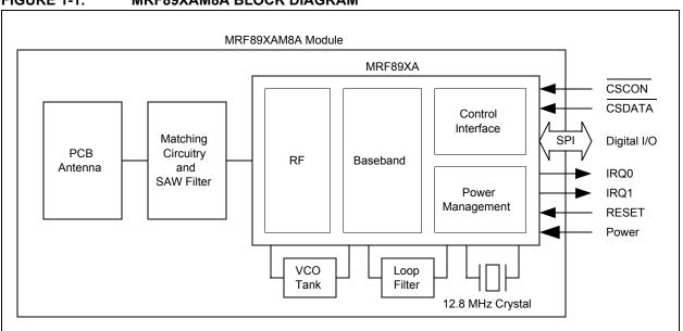
FIGURE 1-1: MRF89XAM8A BLOCK DIAGRAM
