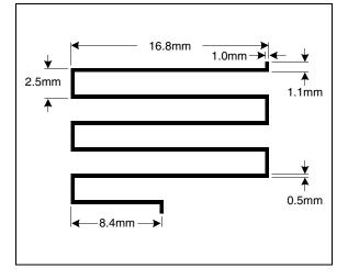
FIGURE 2-11: PCB ANTENNA SIMULATION DRAWING
