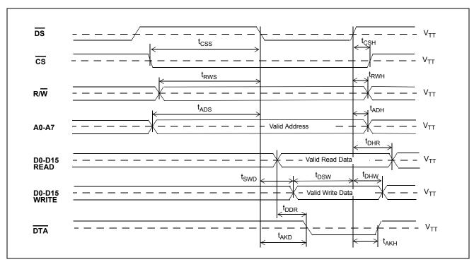
Figure 16 - Motorola Non-Multiplexed Bus Timing
