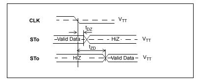
Figure 14 - Serial Output and External Control
