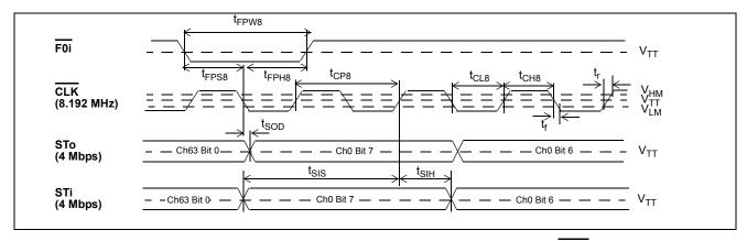
Figure 11 - ST-BUS Timing for Stream rate of 4.096 Mbps when CLK = 8.192 MHz
