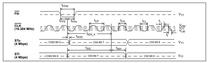
Figure 10 - ST-BUS Timing for Stream rate of 4.096 Mbps when CLK = 16.384 MHz
