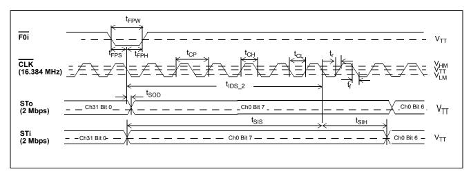
Figure 12 - ST-BUS Timing for Stream rate of 2.048 Mbps when CLK = 16.384 MHz
