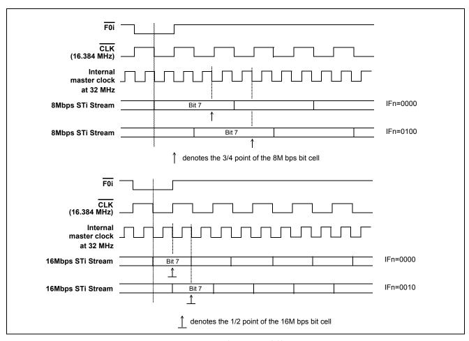
Figure 6 - Examples for Input Offset Delay Timing
