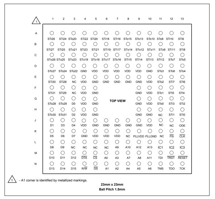
Figure 3 - 160 Ball PBGA Pin Connections
