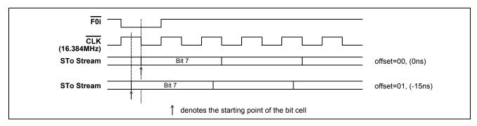
Figure 7 - Examples for Frame Output Offset Timing
