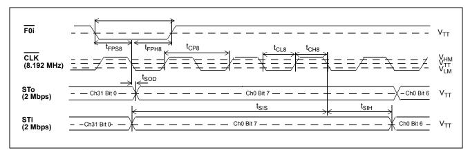
Figure 13 - -BUS Timing for Stream rate of 2.048 Mbps when CLK = 8.192 MHz
