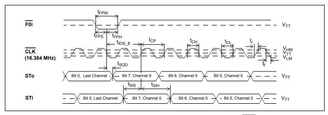
Figure 9 - ST-BUS Timing for Stream rate of 8.192 Mbps when CLK = 16.384 MHz
