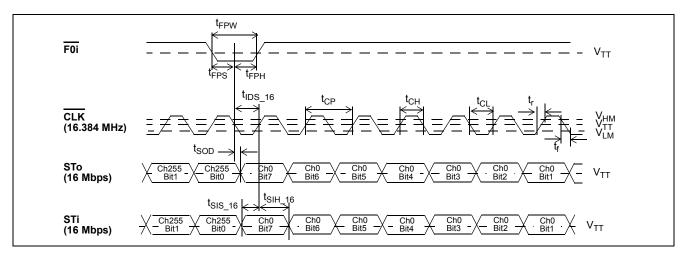
Figure 8 - ST-BUS Timing for Stream rate of 16.384 Mbps
