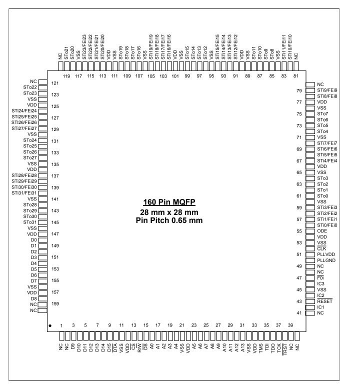
Figure 2 - 160-Pin MQFP Pin Connections
