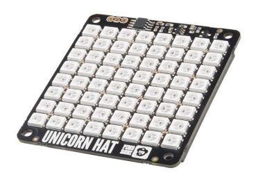
**Description:** The Pimoroni Unicorn HAT is a "shield" for the Raspberry Pi that sports a matrix of 64 (8x8) addressable RGB LEDs that are powered directly from the Pi. The Unicorn HAT provides a wash of controllable color that is ideal for mood lighting, 8x8 pixel art, persistence of vision effects, status indications, or just blasting color into your surroundings.
