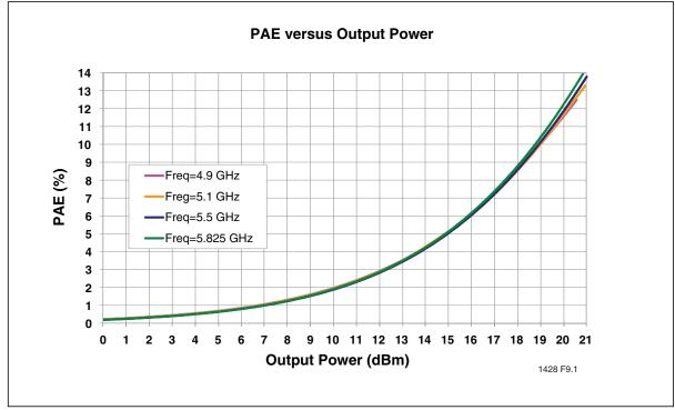
Figure 8: PAE vs Output Power,  $V_{CC} = 3.3V$ ,  $V_{REG} = 2.85$
