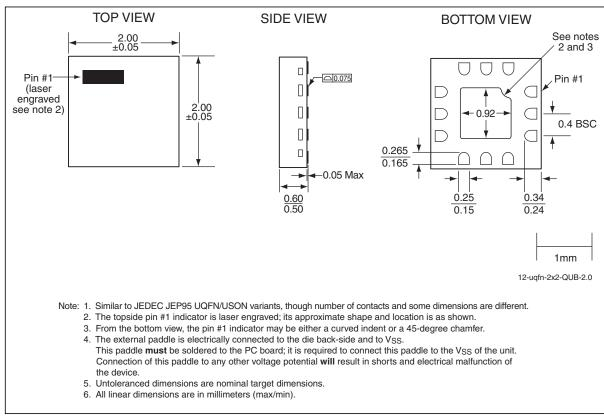
**Figure 15:**12-contact Ultra-thin Quad Flat No-lead (UQFN) SST Package Code: QUB
