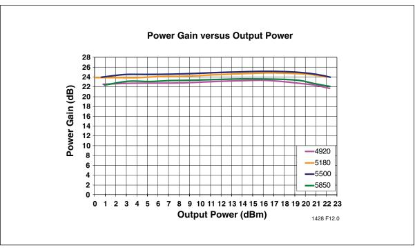
Figure 11:Gain versus Output Power, V<sub>CC</sub> = 5.0V, V<sub>REG</sub> = 2.90V
