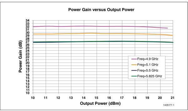
Figure 5: Power Gain versus Output Power, V<sub>CC</sub> = 3.3V, V<sub>REG</sub> = 2.85
