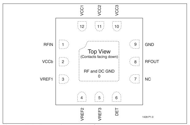
Figure 2: Pin Assignments for 12-contact UQFN
