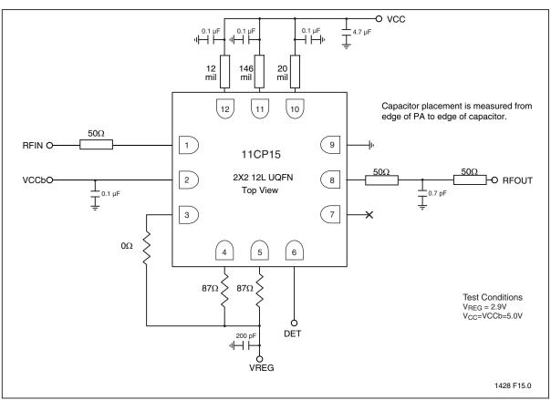
Figure 14:Typical Application for High-Linearity 802.11a/n Application ( $V_{CC} = 5.0V$ ,  $V_{REG} = 2.90V$ )
