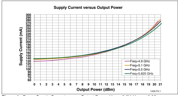
Figure 4: Power Supply Current versus Output Power, V<sub>CC</sub> = 3.3V, V<sub>REG</sub> = 2.85
