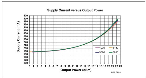
Figure 10:DC Current versus Output Power, V<sub>CC</sub> = 5.0V, V<sub>REG</sub> = 2.90V
