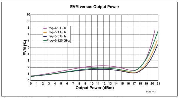
Figure 3: EVM versus Output Power,  $V_{CC} = 3.3V$ ,  $V_{REG} = 2.85$
