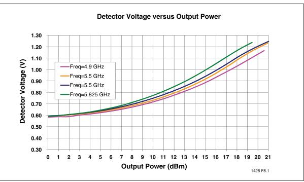
Figure 7: Detector Voltage vs Output Power, V<sub>CC</sub> = 3.3V, V<sub>REG</sub> = 2.85
