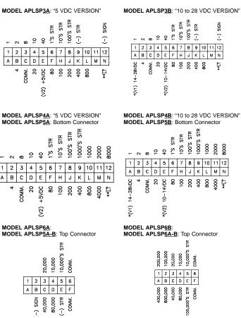
\* Apply power on A and C or E and C.
