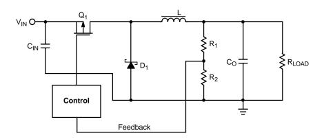
Figure 4. Buck Regulator Block Diagram
