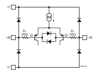
Figure 2. Input Stage Protection
