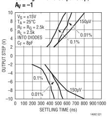
Settling Time vs Output Step,
