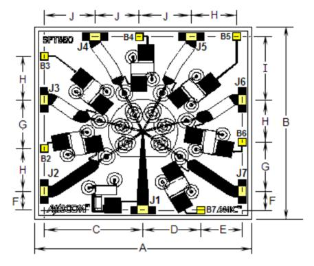
5. Topside and backside metallization is gold , 2.5  $\mu m$  thick typical. 6. Yellow areas indicate wire bonding pads.
