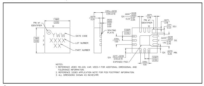
Reference Application Note M538 for lead-free solder reflow recommendations. Meets JEDEC moisture sensitivity level 1 requirements. Plating is 100% matte tin over copper.
