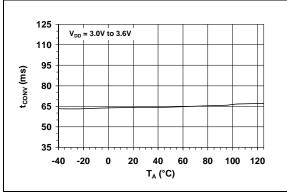
*FIGURE 2-8:* Conversion Rate vs. Ambient Temperature.
