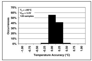
**FIGURE 2-2:** Temperature Accuracy Histogram,  $T_A = +95$ °C.
