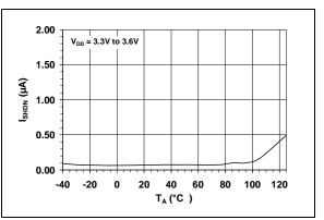
FIGURE 2-5: Shutdown Current vs. Ambient Temperature.
