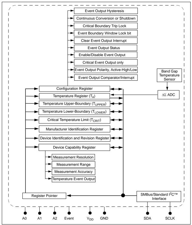
FIGURE 4-1: Register Structure Block Diagram.
