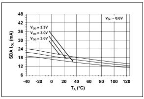
FIGURE 2-10: SDA IOL vs. Ambient Temperature.
