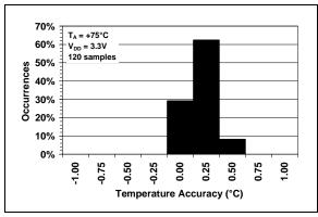
**FIGURE 2-3:** Temperature Accuracy Histogram,  $T_A = +75$  °C.
