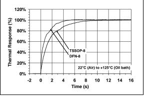
FIGURE 2-12: Package Thermal Response.
