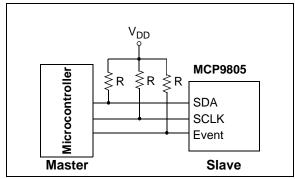
FIGURE 6-1: Pull-up Resistors On Serial Interface.
