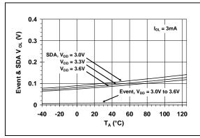
**FIGURE 2-7:** Event and SDA V<sub>OL</sub> vs. Ambient Temperature.
