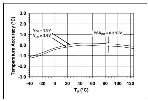
FIGURE 2-11: Temperature Accuracy vs. V<sub>DD</sub>.
