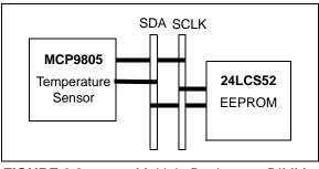
FIGURE 6-2: Multiple Devices on DIMM SMBus.
