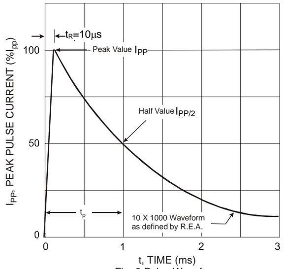
Fig. 2 Pulse Waveform
