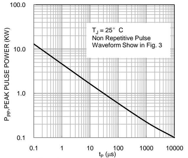
Fig. 4 Peak pulse power versus exponential pulse duration
