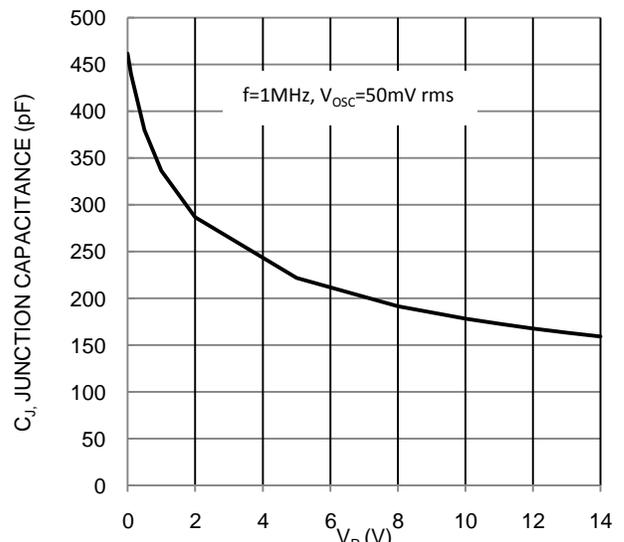
Fig. 6 Junction Capacitance versus Reverse Voltage
