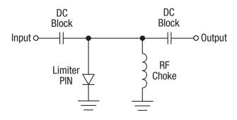
**Figure 2. Single Stage Limiter Circuit**
