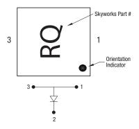
Figure 8. Typical Part Markings (Top View)
