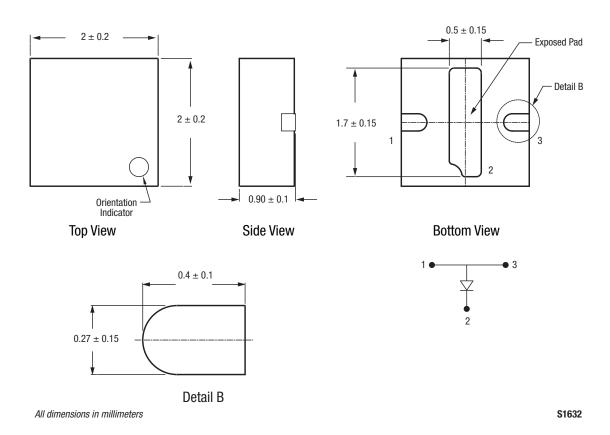
Figure 9. SMP1330-085LF QFN Package Dimension Drawing
