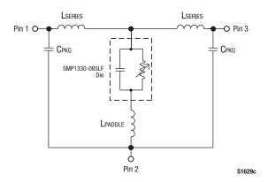
Figure 6. SMP1330-085LF Electrically Equivalent Circuit
