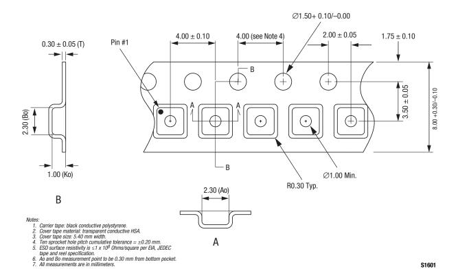
Figure 10. SMP1330-085LF Tape and Reel Dimensions
