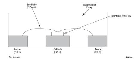
Figure 5. Cross-Sectional View of the SMP1330-085LF
