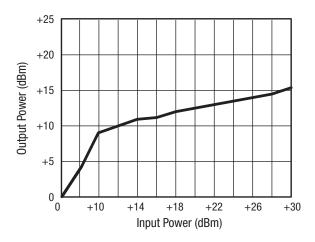
Figure 4. Output Power and Insertion Loss vs Input Power (f = 2.0 GHz)
