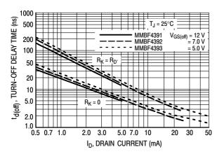
Figure 3. Turn-Off Delay Time
