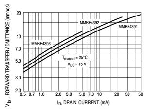
Figure 6. Typical Forward Transfer Admittance
