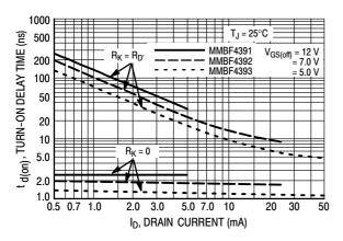
Figure 1. Turn-On Delay Time
