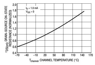
Figure 9. Effect of Temperature on Drain-Source On-State Resistance
