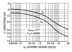
Figure 7. Typical Capacitance
