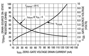
Figure 10. Effect of I<sub>DSS</sub> on Drain-Source Resistance and Gate-Source Voltage
