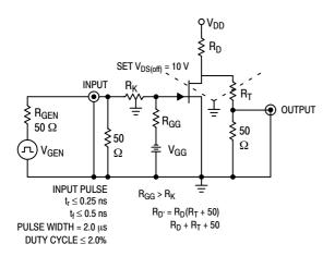
Figure 5. Switching Time Test Circuit
