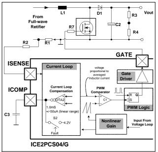
Figure 10 Complete System Current Loop
