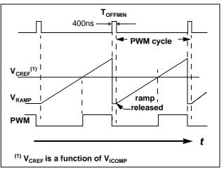
Figure 12 Ramp and PWM waveforms
