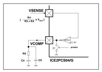
Figure 4 Startup Circuit
