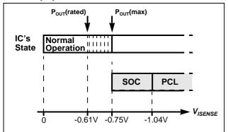
Figure 8 SOC and PCL Protection as function of V<sub>ISENSE</sub>
