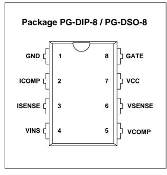
Figure 1 Pin Configuration (top view)
