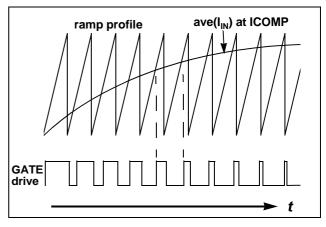
Figure 11 Average Current Control in CCM
