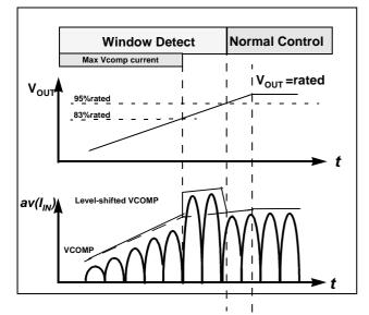
Figure 5 Startup with controlled maximum current
