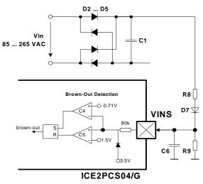
Figure 7 Input Brown-Out Protection (IBOP)
