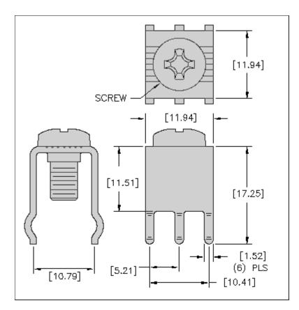
Rated: 30 Amps Terminal: 1.14mm Thick Brass, Tin Plate Screw: M5 x 10mm Thread Combination Binding Head - Brass, Nickel Plate
