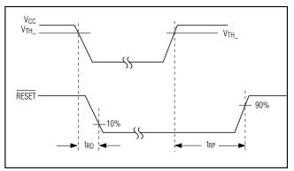
Figure 8. RESET Output Timing Diagram
