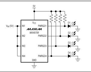
Figure 4. V<sub>CC</sub> Bar Graph Monitoring
