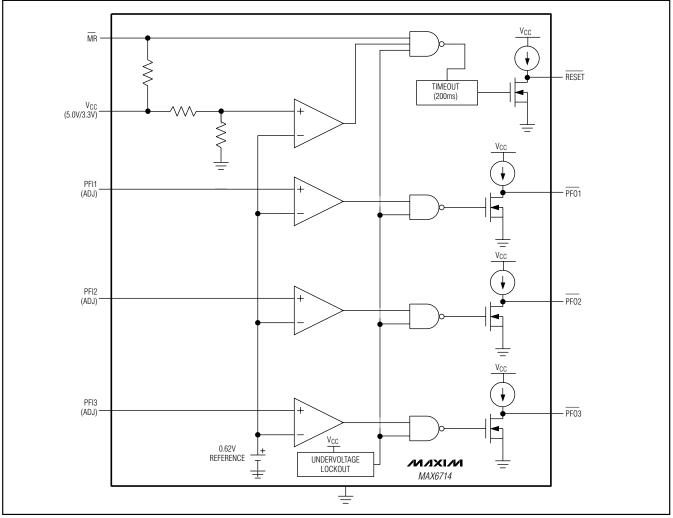
Figure 2. MAX6714 Functional Diagram
