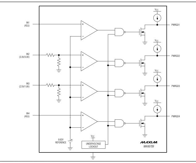
Figure 1. MAX6709 Functional Diagram
