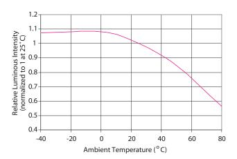
Figure 8. Relative luminous intensity versus ambient temperature.
