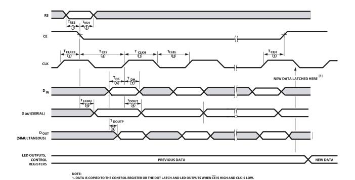
Figure 3. Write Cycle Timing Diagram
