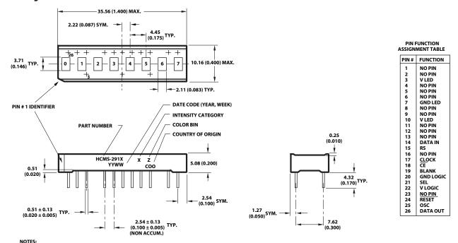
NOTES: 1. DIMENSIONS ARE IN mm (INCHES). 2. UNLESS OTHERWISE SPECIFIED, TOLERANCE ON DIMENSIONS IS  $\pm$  0.38 mm (0.015 INCH). 3. LEAD MATERIAL: SOLDER PLATED COPPER ALLOY.
