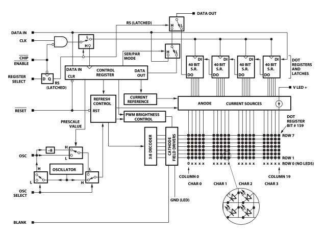
Figure 5. Block diagram
