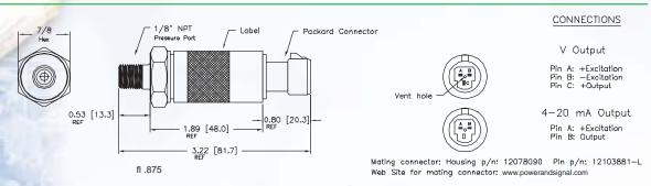
Vent through hole in connector ( under 1000 psi ) Add 0.4" for CE EMI/RFI protection. Note: Mating connector is available with 3 ft of cable PN (2001140).
