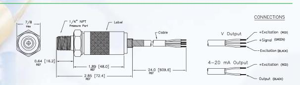
Vent through cable ( under 1000 psi ). Add 0.4" for CE EMI/RFI protection, max operating temperature for cable is 100°C.
