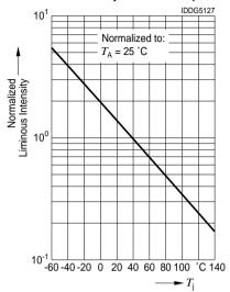
When mounted in a 10°C/W socket and operated at Absolute Maximum Electrical conditions, the display will show an LED junction rise of 17°C. If  $7_{\rm A}$ =40°C, then the LED's  $7_{\rm J}$  will be 57°C. Under these conditions the following Figure "Max. LED Junction Temperature vs. Socket Thermal Resistance" shows that the  $I_{\rm V}$  will be 75% of its 25°C value.
