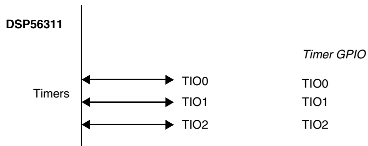
Figure 5-6. Triple Timer Signals
