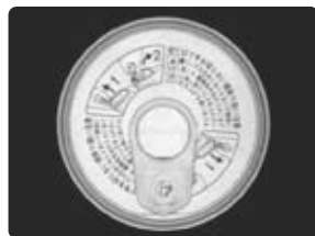
With radiation from LWD 10mm, it can capture the object uniformly without convex-concave.
