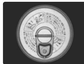
With radiation from LWD 85mm, the convex-concave of the pull-tab part is emphasized.
