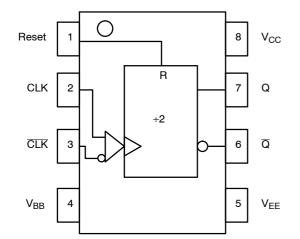
Figure 1. Logic Diagram and Pinout Assessment
