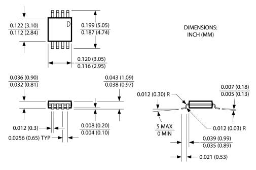
8-Lead MSOP (MM)
