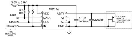
2-Channel SMBus Temperature Measurement System
