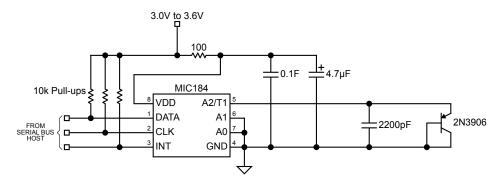
Figure 9.  $V_{\mbox{\scriptsize DD}}$  Decoupling for Very Noisy Supplies
