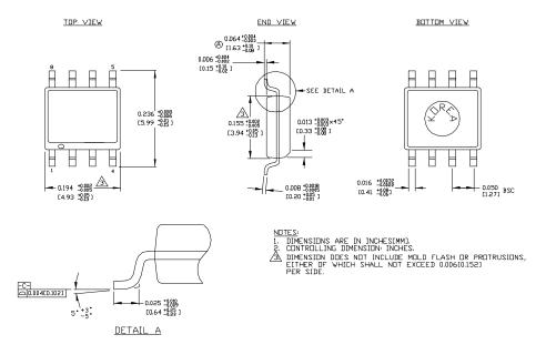
8-Lead SOIC (M)
