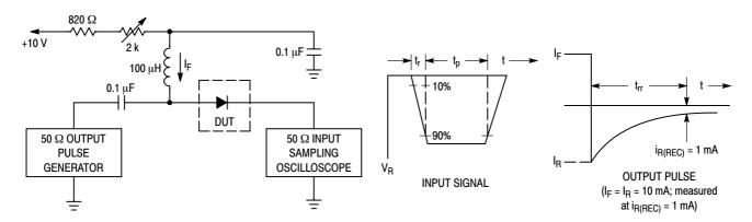
Notes: (a) A 2.0 k $\Omega$  variable resistor adjusted for a Forward Current (IF) of 10 mA.
