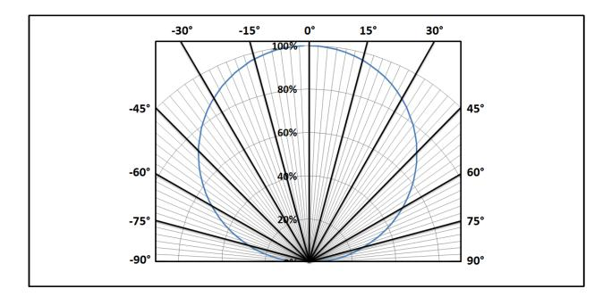
Figure 7: Typical Polar Radiation Pattern
