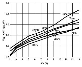
FIGURE 10. DIGITAL SWITCHING POINT vs SUPPLY VOLTAGE
