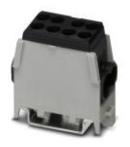
Trunk line branch terminal, Connection method: Screw connection, Screw connection, Number of connections: 4, Number of positions: 1, Cross section: 1.5 mm<sup>2</sup> - 25 mm<sup>2</sup>, AWG: 8 - 2, Width: 23 mm, Color: black, Mounting type: NS 35/7,5, NS 35/15
