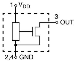
Fig. 4–1: Pin configuration
