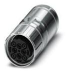
Cable connector, straight long, Screw locking, M40, Number of positions: 4+3+PE, Type of contact: Socket, Crimp connection, Shielded: Yes, Cable cross section: 20.5 mm...26.5 mm
