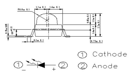
**Notes:** 1.All dimensions are in millimeters 2.Tolerances unless dimensions ±0.1mm
