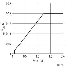
Figure 4. Dimming and Shutdown Using CTRL Pin
