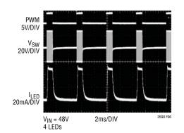
Figure 6. Direct PWM Dimming Waveforms
