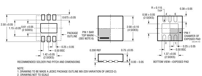
DC Package 6-Lead Plastic DFN (2mm × 2mm) (Reference LTC DWG # 05-08-1703)
