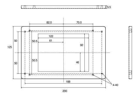
Material : Steel Finish : Grey Powder Coat Dimensions in mm
