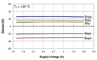
Switch Points vs Supply Voltage
